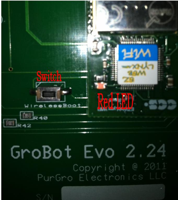
Unplug the 'Bot. Hold the switch down and power the 'Bot back up, holding the switch down until the LED on the WiFi radio lights up (about 5 seconds).
