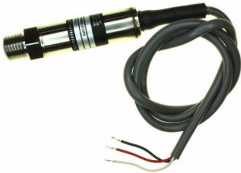
The BEST way to do this is to drill a hole in the side of the res and install a bulkhead fitting with ½” NPT threads. Screw the sensor into the fitting and tighten it down. If that’s not possible, you can Tee it into your drain line. The sensor measures the WEIGHT of the water column as pressure, and requires no setup or calibration.
